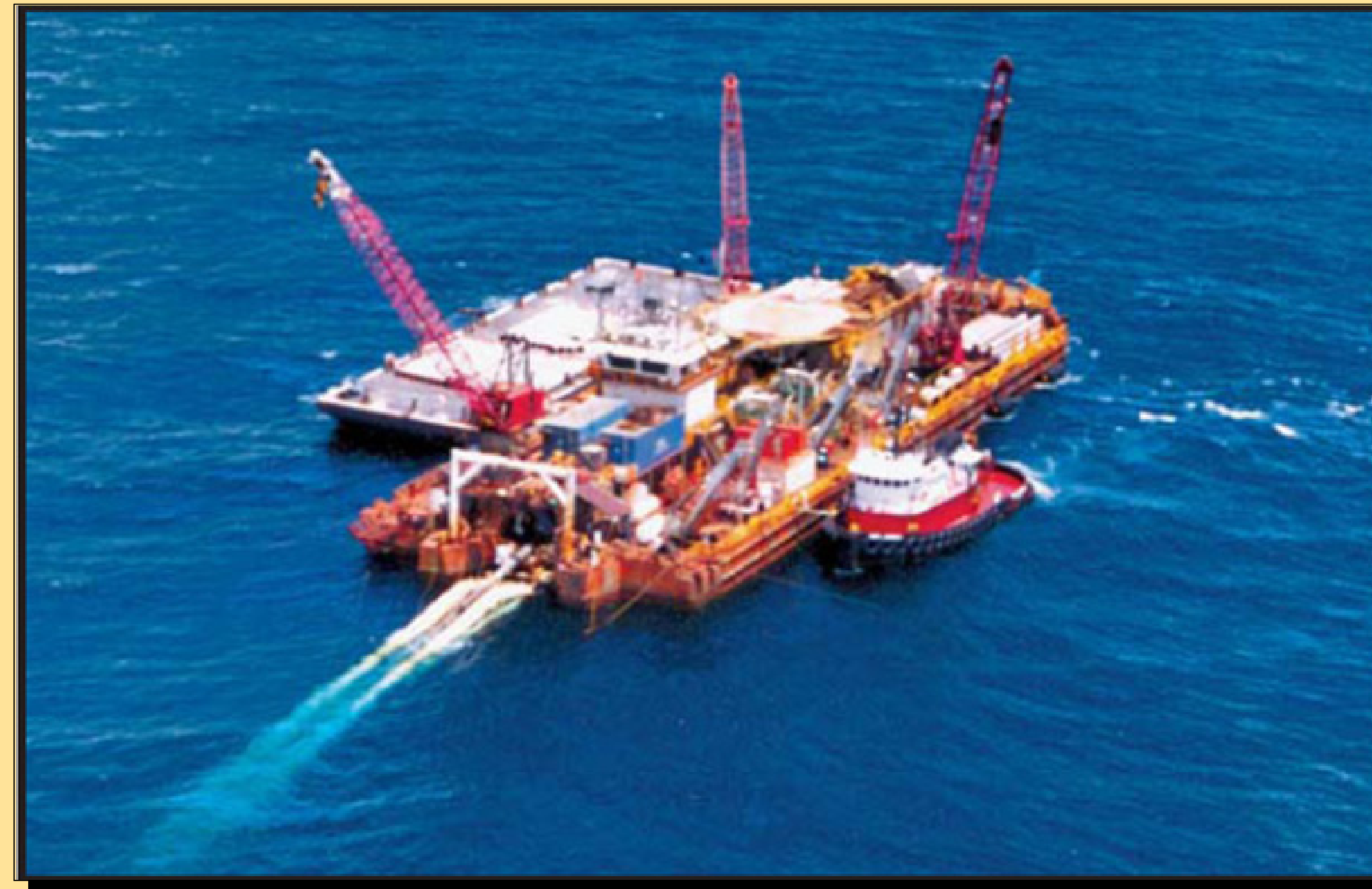
Typical Lay Barge
