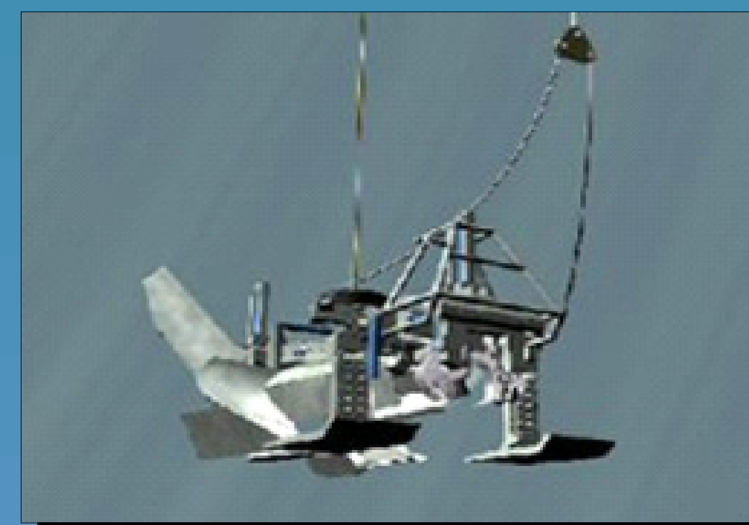
Plow being lifted into position over pipeline
