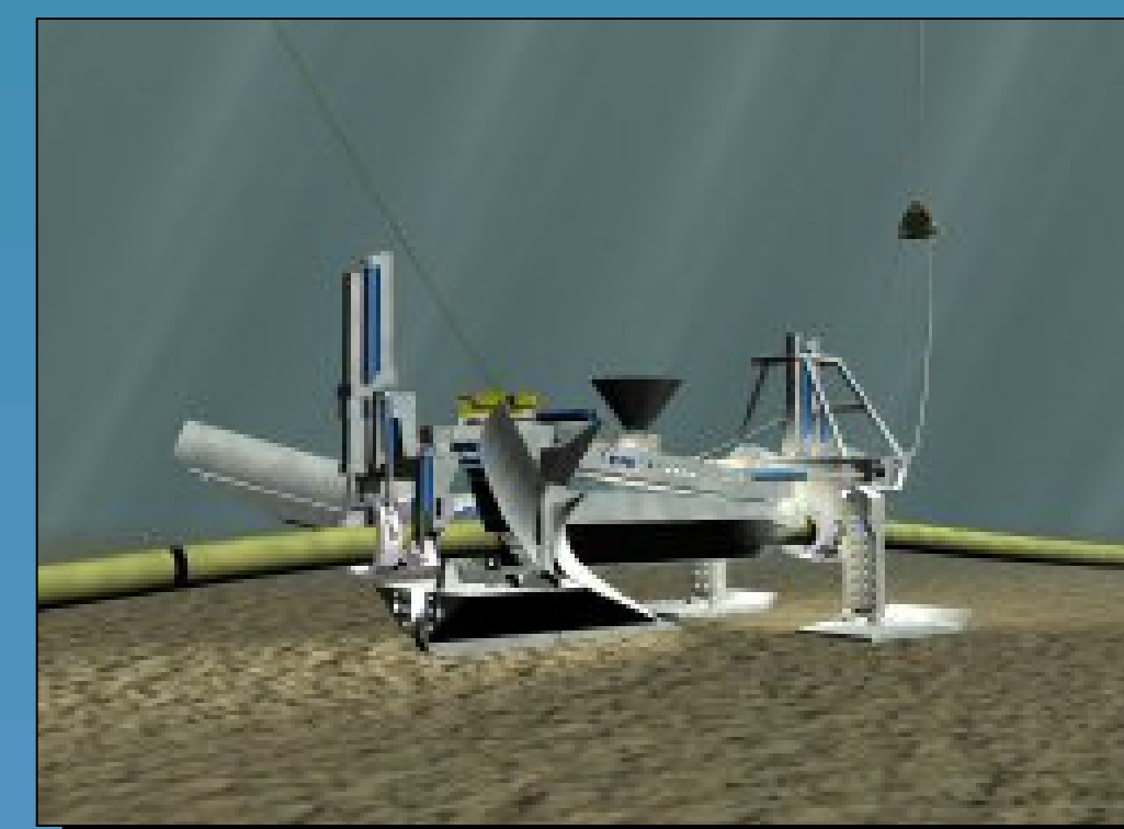
Plow cradling the pipeline at the start of the plowing process
